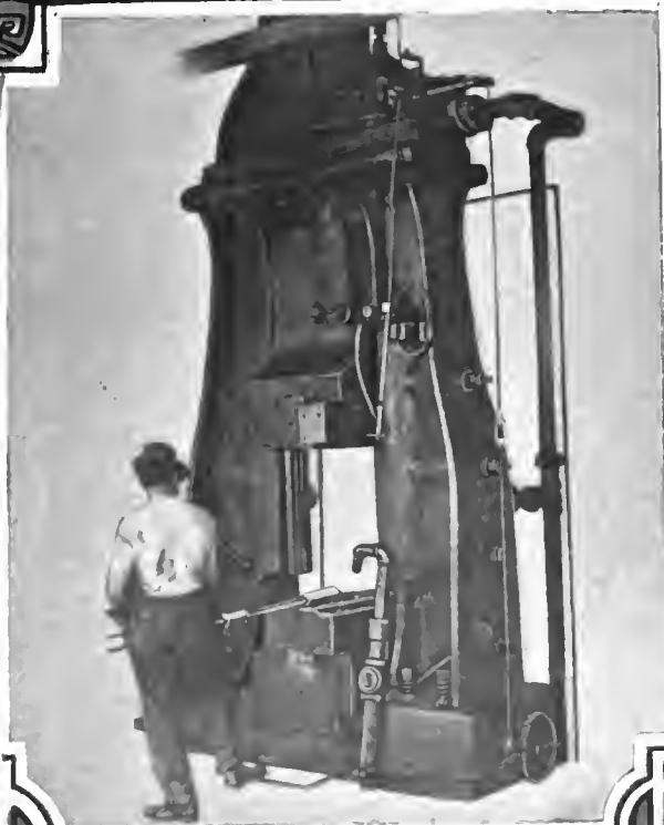
B—Heavy Press in the Act of Drop-forging a Special Steel I-Section Front Axle, Showing How the Bar of Steel Is Placed on the Breaking-down Die and Given Its Preliminary Shape
